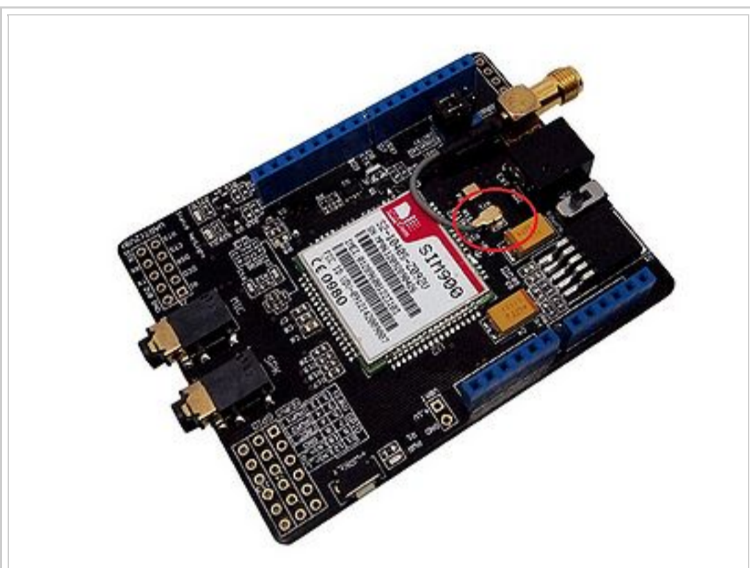
Antenna pad properly buckled
