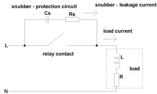
Connection of the snubber circuit in parallel to the switch
