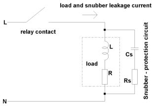
Snubber circuit connected in parallel to the load
